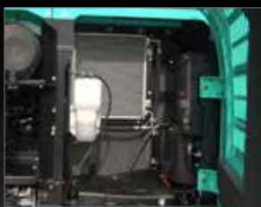
Left side (radiator and cooling system elements)
