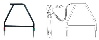
The vLoc3 series A-frame accessory is used to detect ground faults on pipes and cables. In the case of pipes, the faults consist of coating defects. In the case of cables, faults are usually caused by insulation damage allowing the metallic sheath (or internal conductor) to become in contact with the ground.
