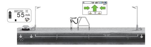
Plug in the analogue A-frame to the receiver accessory socket. When the receiver is switched on, it will automatically default to the A-frame screen.
