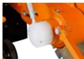
Water cooling through the blade shaft
