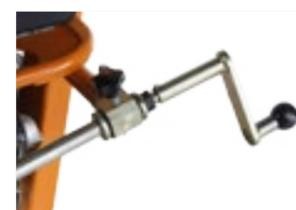
Cutting depth adjustment by handwheel
