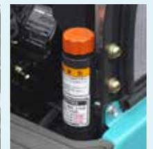
Long-life hydraulic oil with a replacement cycle of 1,000 hours (Photo shows the hydraulic oil port.)
